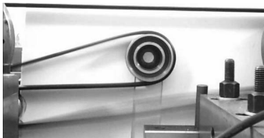
Fig. 2 Example of instability in slack belt span
